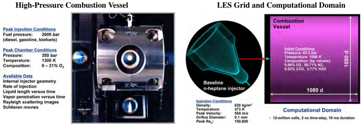
**Figure 4:** Photograph of the Sandia high-pressure combustion vessel (left) and computational domain used for LES (right). The injector is mounted at the head-end of the vessel, as indicated by the red arrow.
