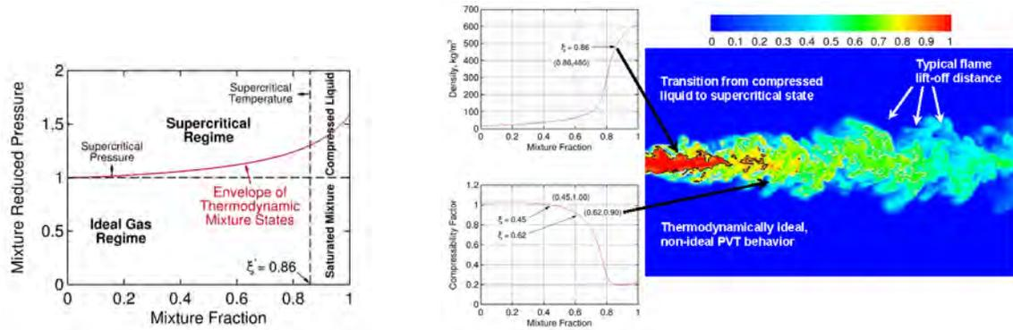
**Figure 6:** Envelope of mixture states predicted as a function of mixture fraction  $\xi$  (left) and contour plot showing a representative LES prediction of mixture fraction (right). Iso-lines mark the transition of the mixture from a compressed liquid to supercritical state (black) and separation between regions of non-ideal and ideal fluid behavior (white).
