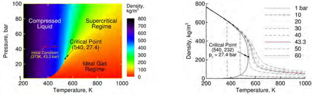
**Figure 5:** Thermodynamic characteristics of n-heptane showing key regimes and its initial state when injected. N-heptane enters as a compressed liquid and is heated at supercritical pressure.
