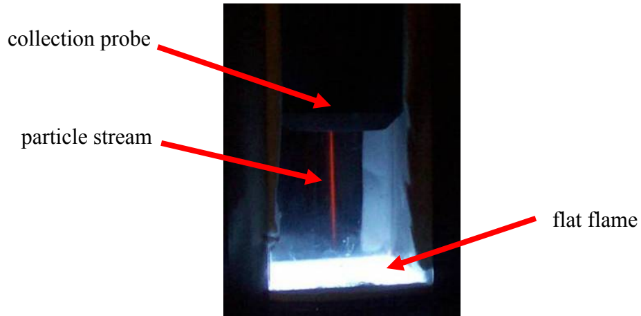
Figure 3. Biomass particles being pyrolyzed in the FFB reactor.
