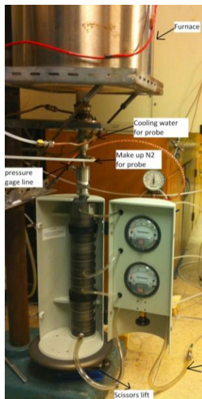
Figure 1. Photo of the experimental set-up consisting of electrically-heated laminar-flow drop-tube furnace coupled with the 13-stage Nano-Moudi ash particle impactor through a dilution N_2 probe.
