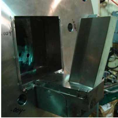
Figure 1 Photograph of the HEAT injector integrated flame holder assembly and mounting flange.
