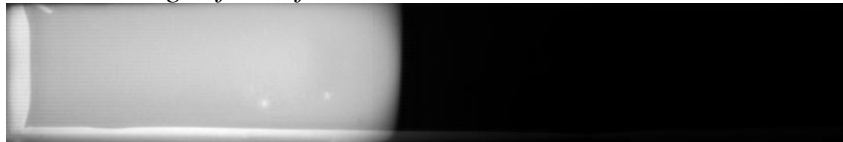
t=30 ms: Planar flame front appears.
