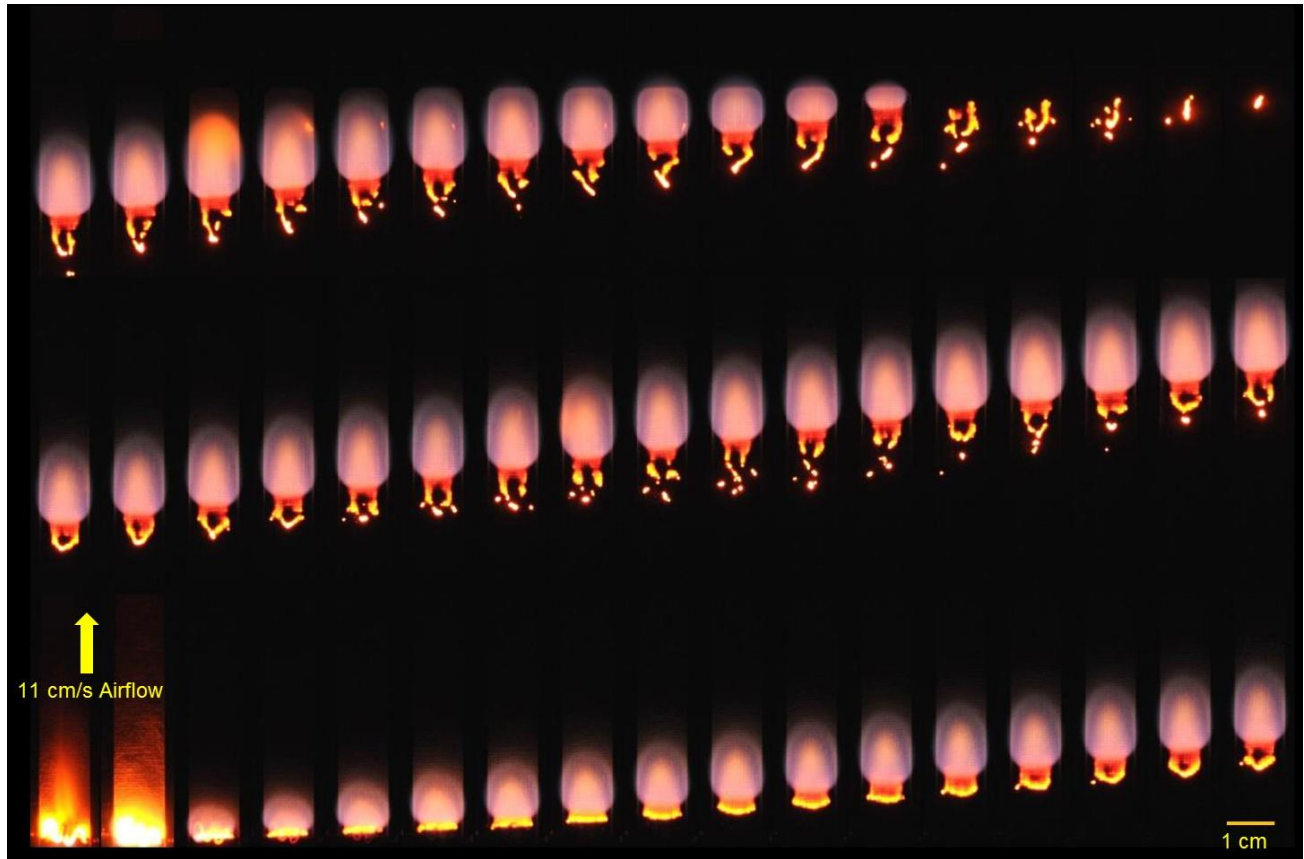
Figure 10. Digital still camera images for 1-cm-wide fuel with concurrent air flow = 11 cm/s. Images are taken every 1.125 sec (starting at bottom and moving from left to right). The flame reaches steady state after about 10 seconds. (Test 10)
