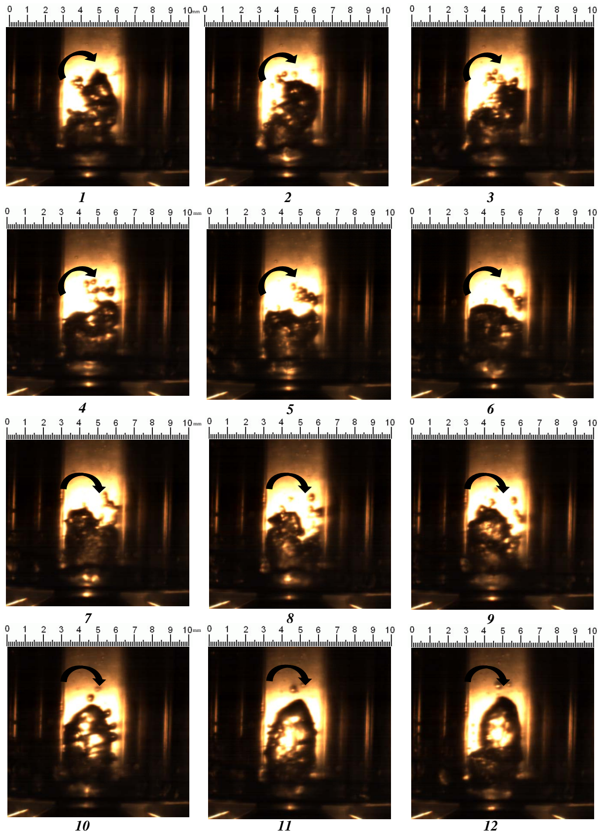
Figure 15. Bubble Dynamics illustrated by images taken 1 ms apart, ALR = 2.04
